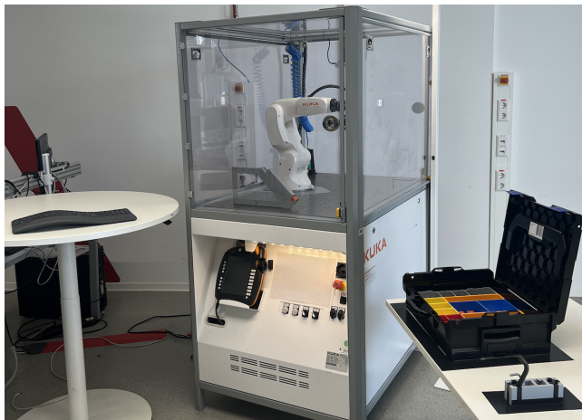
Figure 3: The setup used for the authoring study consisted of a table with a keyboard, a KUKA Ready-2-Educate robotic cell, and a workplace with materials and tools needed.
