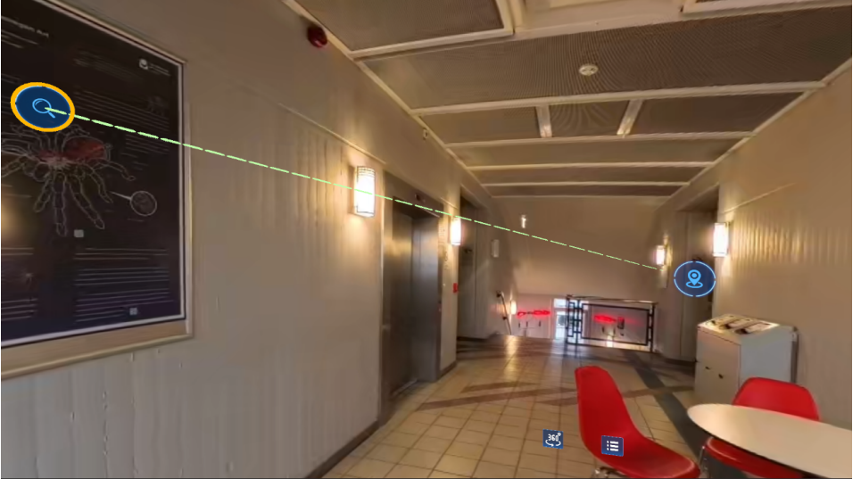
Fig. 1: Selection with Item Scanning: Interactive elements are sequentially highlighted. The highlighted element can be selected by pressing the switch
