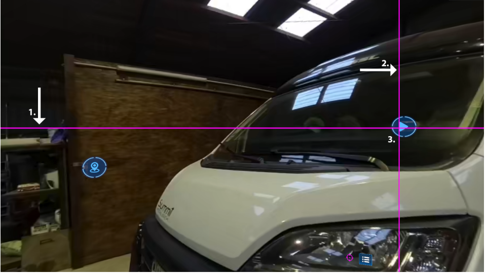
Fig. 3: Selection with Cartesian Scanning: (1) first Scanning Line moves from top to bottom, (2) second Scanning Line moves from left to right, (3) intersection point is used for selection
