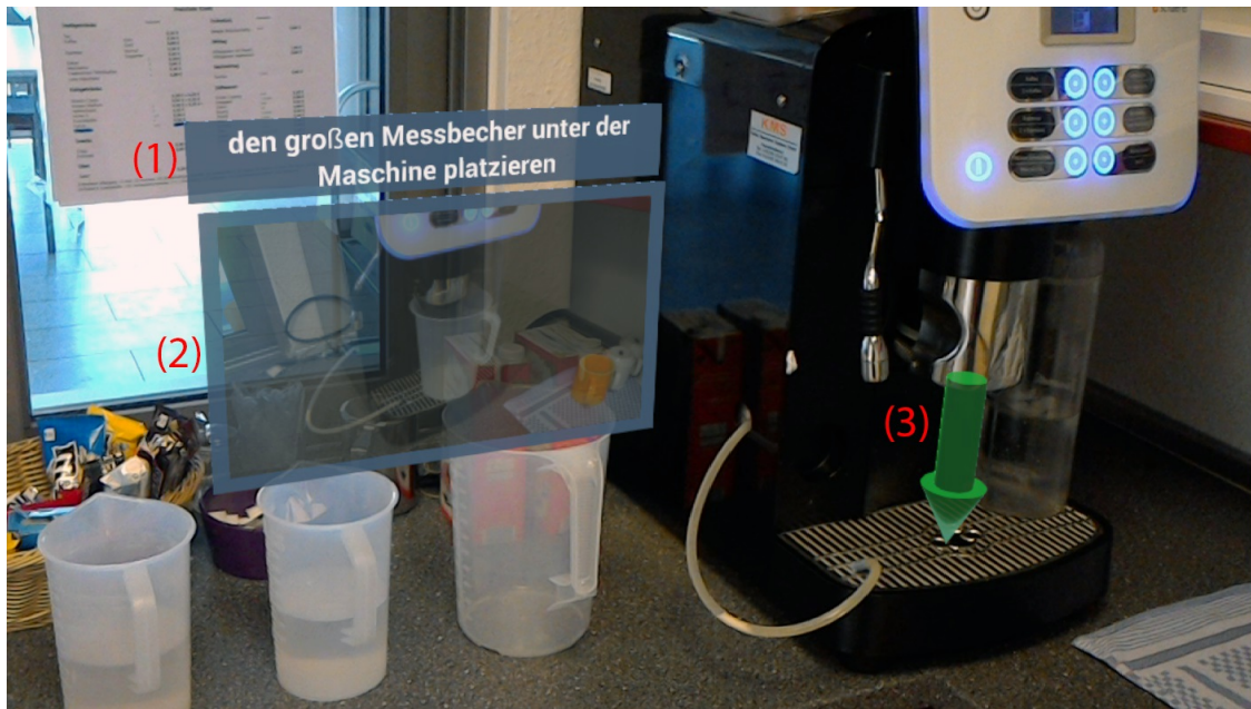
Figure 1: The AR instructions displayed on the MS HoloLens. Multiple types of instructions were combined for each step: (1) text instructions, (2) photos (e.g. taken from the the target state) and (3) in-situ arrows indicating the physical position.
