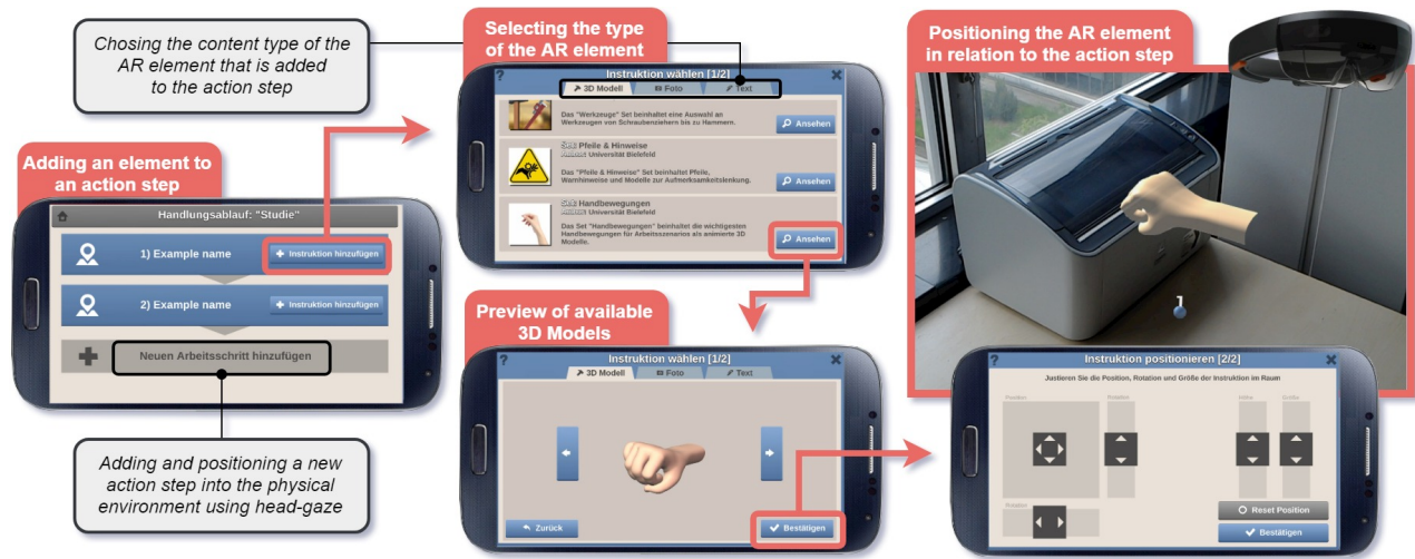
Figure 3: Practical example: The process of adding an AR element (hand animation) to an existing action step (1), that shows how to open the paper lid of a printer, using the authoring tool.
